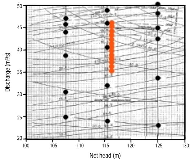
Fig. 14 - Log of the model tests of the turbines presented in Figs. 1-9: the black dots stand for model tests and the red dots for the multidimensional monitoring results. The latter cover the whole range of a normal operation. Thus, only two model points are directly useful in practice.
