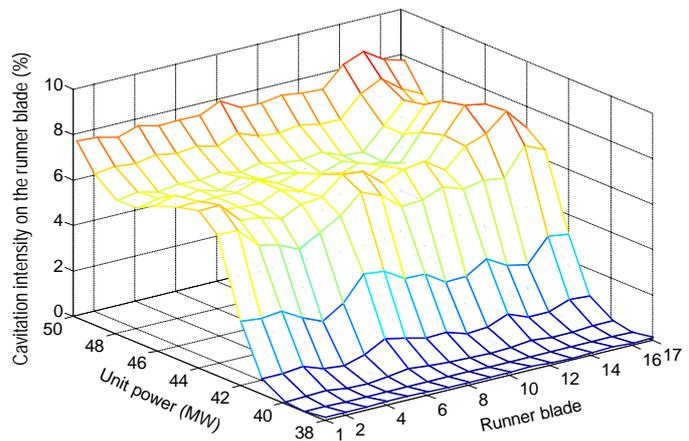
Fig. 3 - **Wicket-gate cavitation characteristic** reflects both differences in wake-fields behind individual vanes, i.e. their cavitation-related quality, and the differences in the flow conditions behind different parts of the spiral casing. Here, the second effect is dominant.
