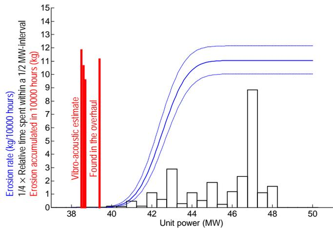
Fig. 6 - This *special form of the global cavitation characteristic* yielding cavitation intensity in the draft tube shows that the Unit B, which has lower intensity of the erosive cavitation (Fig. 4), has stronger cavitation below the runner, in the draft tube. This shows that the stability in the partial-load operation of Unit B must be checked.
