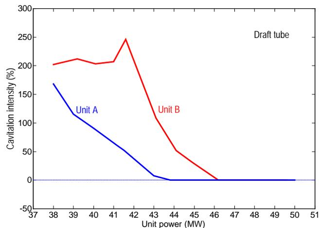
Fig. 7 - Well-interpreted rich data on cavitation delivered by the multidimensional monitoring enables **recognition of the cavitation mechanisms** and their quantitative assessment. In the group of this and two subsequent graphs the result of such a procedure is presented. The basic format, as in Fig. 3, is used to present three components of the total intensity, which stem from three cavitation mechanisms related to the runner. In this figure, the erosive areal cavitation is quantified.
