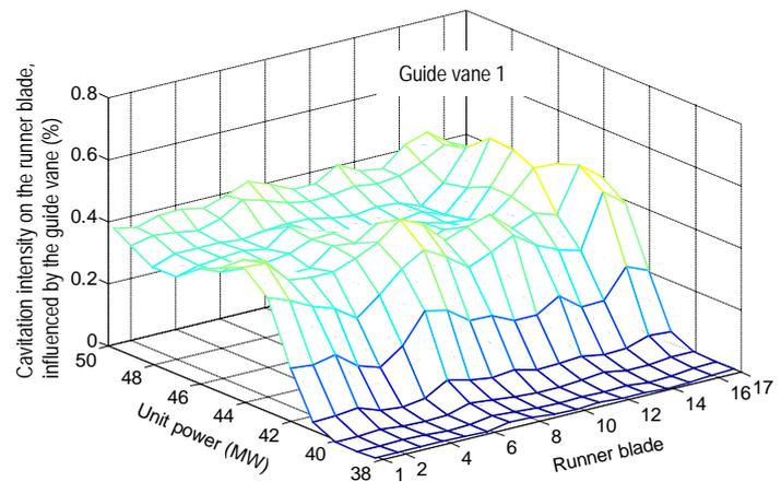
Fig. 2 - **Runner cavitation characteristic** assesses the average cavitation quality of each runner blade, i.e. its quality averaged over all the wicket vanes. In this case, there are no large differences among the blades.
