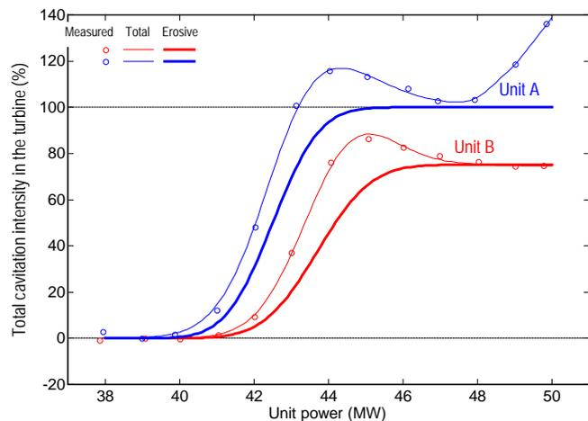
Fig. 5 - *Absolutely calibrated global cavitation characteristic* yields erosion rate for different operation conditions. By combining this vibro-acoustic data (accompanied by the uncertainty bounds) with the planned loading statistics for a future period, the accumulated erosion in that period can be predicted. This enables optimisation of the maintenance schedule.
