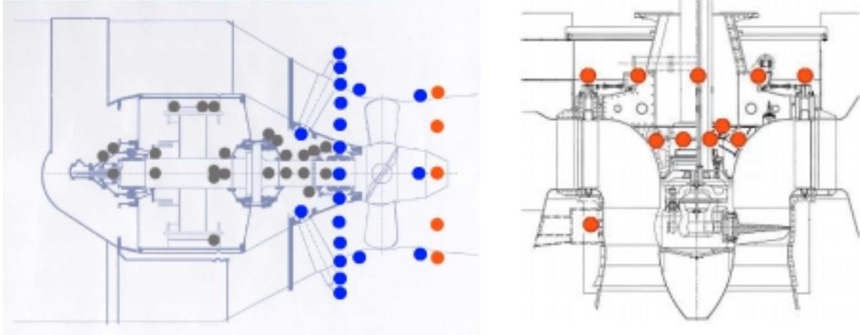
Fig. 11 - Examples of sensory systems. A large number of sensors is used in a cavitation diagnostic test (blue and red dots). Only a part of them is used for permanent monitoring of cavitation (red dots). The other dots at the bulb unit denote various other sensors used in a general monitoring system.
