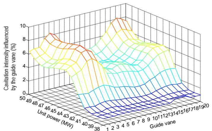
Fig. 4 - *Global cavitation characteristic* yields the simplest description of cavitation in a turbine. By comparing all units in one plant in respect to the differences as found here (the cavitation intensity on Unit B is 25 % lower than on Unit A, and the cavitation starts at 1 MW higher loading), an operation plan can be made to minimise the total erosion. Usually, the characteristics vary more than these two, which makes such optimisation even more efficient.
