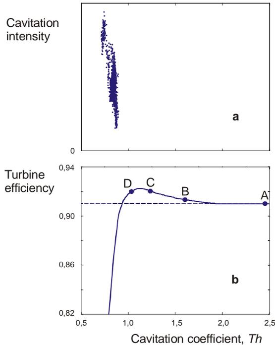
Fig. 10 - Results of full-scale vibro-acoustic tests of the cavitation intensity dependence on the cavitation coefficient in Dubrava turbine A (a), and model-scale results on the cavitation influence on the turbine efficiency for Dubrava at the head and discharge close to the nominal values [15] (b)
