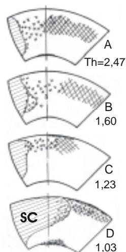
Fig. 9 - Cavitation forms close to the nominal head and discharge values as found in model tests for the Dubrava turbines at four values of the cavitation coefficient,  $Th$  [16]. Various types of cavitation present vary in erosion intensity; sheet cavitation (SC) is not particularly dangerous.
