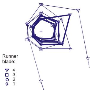
Fig. 6 - Cavitation intensity close to each of the 4 runner blades (radial coordinate) in relation to the instantaneous runner angular position described by the position of the blade 4 (angular coordinate) [13]: thick lines – weak fluctuations, thin lines – strong power fluctuations.
