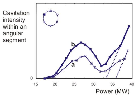
Fig. 7 - Influence of the incorrect guide blade position [13] – cavitation intensity in the angular segment behind a blade which is open for  $5^\circ$  more than needed: (a) normal position of the blade, (b) incorrect position.
