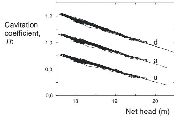
Fig. 11 - Survey of the Dubrava operating conditions: cavitation coefficient at the axis (a) and on the runner blade top when it is down (d) or up (u), in relation to the net head, for a typical head water
