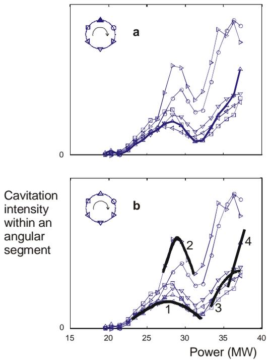
Fig. 4 - Cavitation intensity in 6 angular segments of the turbine denoted by 6 different symbols (downstream view; the arrow denotes rotation direction) [13]. In figure **a** the upper angular segment with the lowest pressure is marked by the solid line, and in figure **b** traces of four cavitation mechanisms appearing in the turbine are shown.
