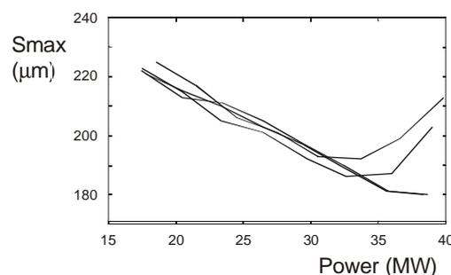
Fig. 16 - Shaft vibration amplitude of the Dubrava unit A downstream of the axial bearing at four different conditions [11].
