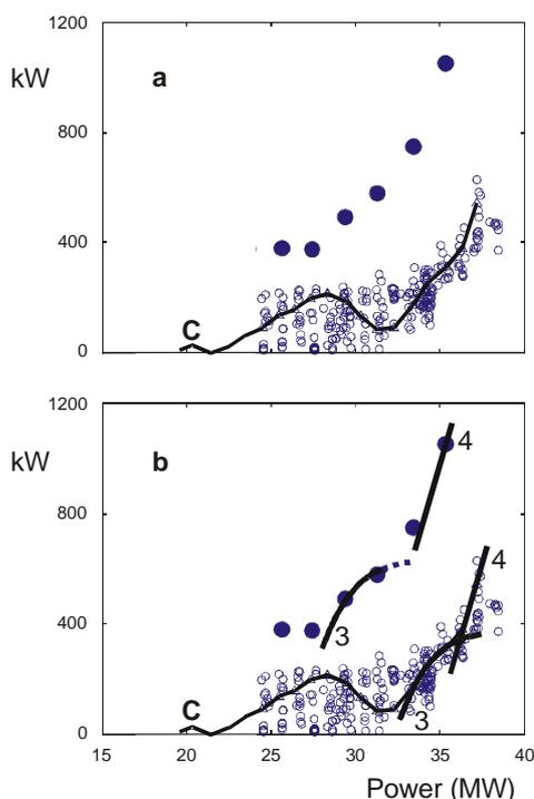
Fig. 8 - Data on the power-dependence of the power fluctuations amplitude (from Fig. 2) compared with the data on the power-dependence of the cavitation intensity:
