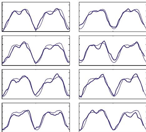
Fig. 14 - Waveform of the instantaneous power deviation from the mean value found in the case of strong fluctuations in 8x2 subsequent revolutions: thick line – measured, thin line – simulation result
