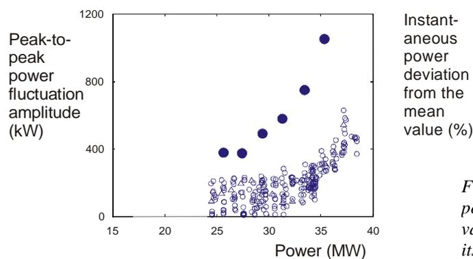
*Fig. 2 - Measured power-dependence of the periodic component of the deviation of the instantaneous power from the mean value: hollow dots – weak fluctuations, solid dots – strong fluctuations.*
