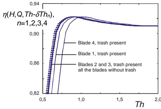
Fig. 12 - Cavitation quality of the runner blade assessed by means of vibro-acoustic cavitation intensity estimates; the best blade is assumed to follow behaviour found by the model testing.
