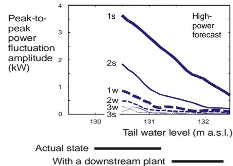
Fig. 15 - Assessment of the runner quality regarding power fluctuations at high power values and a typical head water:
