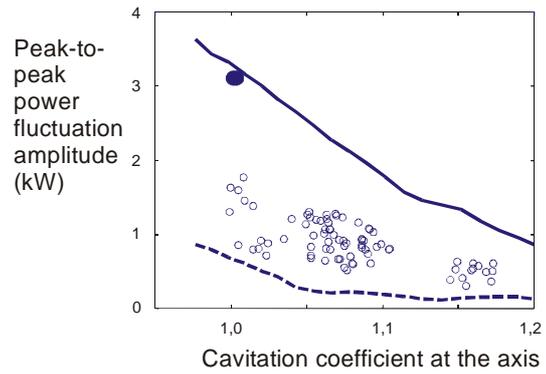
Fig. 13 - Simulation results (lines) and measurements (dots): the solid line and the solid symbol – strong fluctuations (trash on the guide vanes acts); the broken line and the hollow symbols – weak fluctuations (without trash). This description is valid for high power values at the head close to the nominal one.
