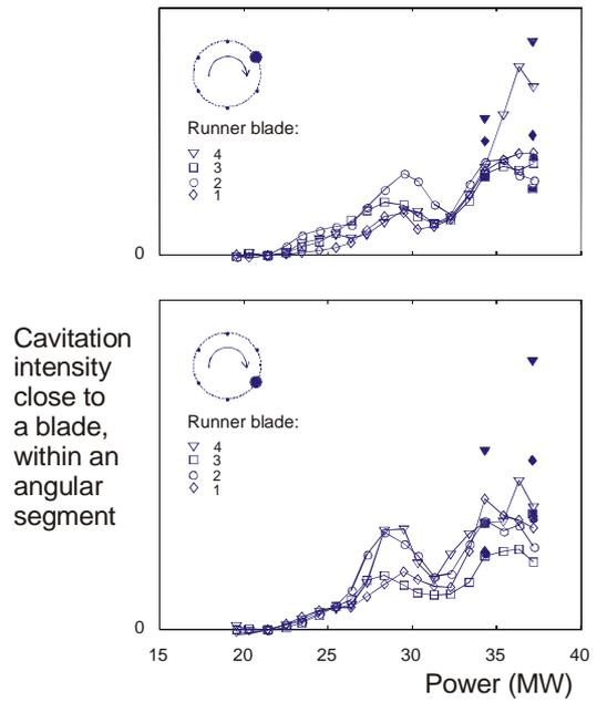
Fig. 5 - Cavitation intensity close to each of the 4 runner blades in two angular segments – upper right and down right [13]: hollow symbols and lines – weak fluctuations regimes, solid symbols – strong fluctuations regimes.
