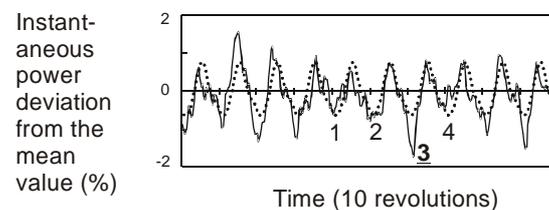
*Fig. 3 - A typical waveform segment of the power fluctuations recorded at a high power value (solid line) and the approximation of its deterministic, slowly varying component (dots)*
