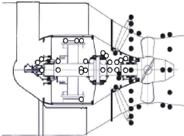
*Fig. 1 - Dubrava HPP unit A with sensors used in the multidimensional diagnostic tests. In the diagnostics of cavitation and power fluctuations the sensors marked by solid dots and sources of data on operating conditions were used.*
